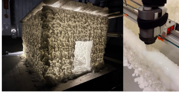
Figure 2: The final printed rigid walled structure made of high performance ice composite (left). The structure was arbitrarily completed at approximately 3'x'2'x'2' dimensions. A line of ice slurry deposited during operations (right).
